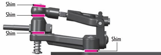
Front ride height can be adjusted by placing shims at various locations on the kingpin and also under the front lower bulkhead. Ride height is influenced by the tire diameter. The amount of shims has to be the same on both left and right sides.
